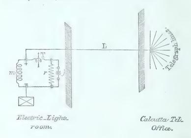
J represents an electric light, in this case produced by a large Serrinlamp.
